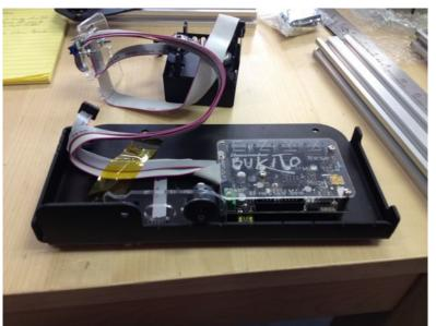
Attach the acrylic piece with the power switch to the baseplate assembly using the screw and square nut and shortest of the screws in this kit.
