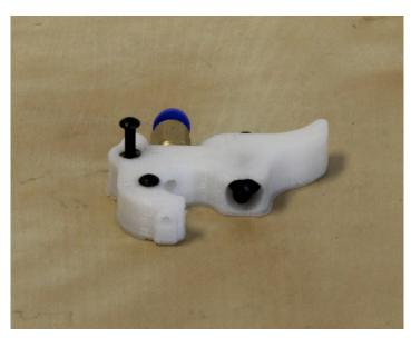
Drop screw and spring into the hole in the part with the blue flange. (Hole is in front of you – screw point is facing out.)
