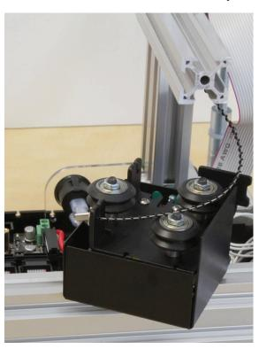
Take the extruder carriage and slide it onto the x axis, being careful to place the wheels over the synchromesh. Then hook the synchromesh into the tabs on the bottom of the X carriage.
