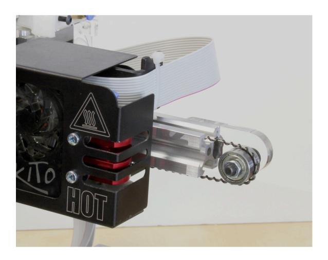
Take the x end stop kit and put the acrylic cover over the circuit board, aligning so that the protruding parts of the board are in the cutouts.
