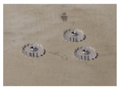
Take the platform and connect it to the carriage as shown. Hold the platform down with one hand and tighten the screws (using the "flowers") as much as you can. You will back it off later to adjust it.
