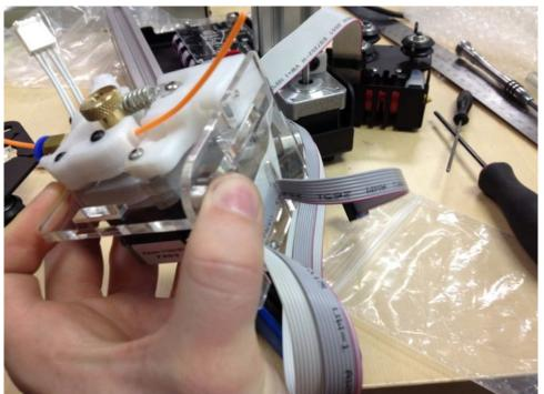
Plug motor into circuit board on assembly.
