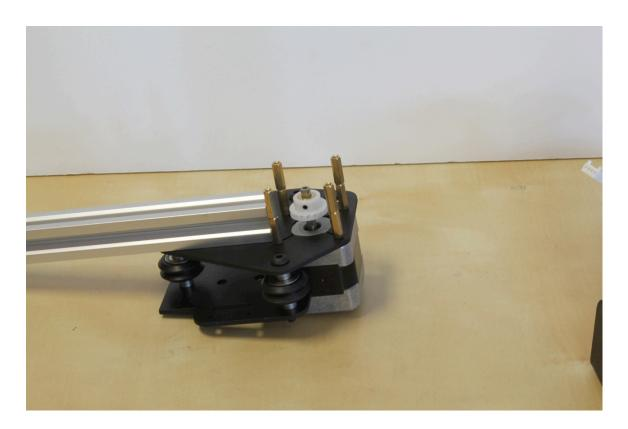
Take shorter of the two pieces of synchromesh and be sure there is a washer on either end. Put the mesh in the valley of the top of the x carriage aluminum bar.
