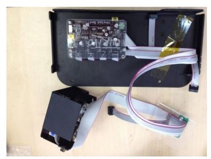
Gather up the main assembly (baseplate, control board and extruder, with cables) and the two aluminum 11 inch extruded rods.
