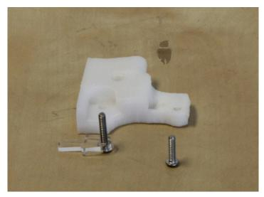
Open the extruder drive mechanism kit. Be sure not to lose the small piece –the spring (a few steps down) hooks over the narrow part of this small acrylic piece.
