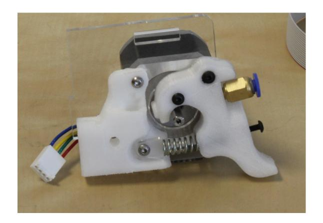
Put filament in to check drive gear alignment. Motor connector should be on same side as blue flange.
