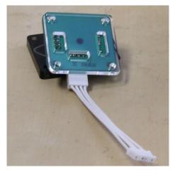
Take the x end stop kit and put the acrylic cover over the circuit board, aligning so that the protruding parts of the board are in the cutouts. Attach the part with the Bukito logo to the other side (facing away from you in this photo.) Be sure to take the brown paper backing off the Bukito logo acrylic piece.
