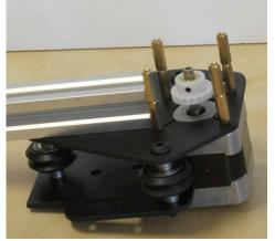
Align the syncromesh pulley (white plastic part) with slot of the extruded aluminum rod. Once it is aligned, rotate the pulley so that the small screw on the side (dark spot on side in image) is on the flat part of the motor shaft so that it can be tightened down. Use a 1.5mm allen wrench. Be sure it is solidly tightened or you will get a lot of backlash when printing if the pulley is loose.
