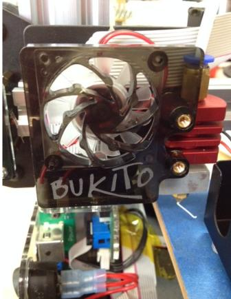
Next, clip the original fan back into place over the extruder. Then put the metal cover back and finally the new acrylic. Use the new screws included in the fan kit.
