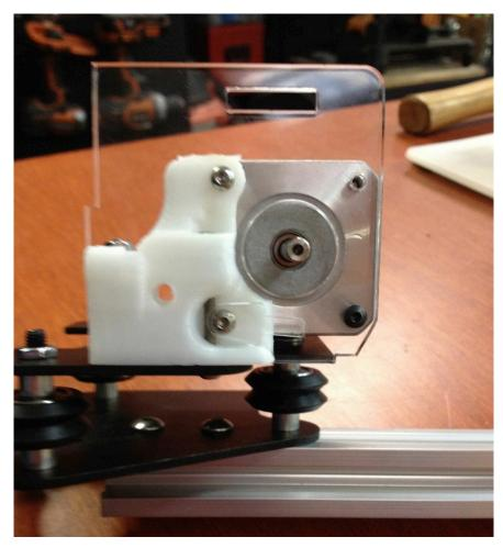
Take the white acrylic piece without the blue flange and attach it to the x axis and carriage using the long screws provided.
