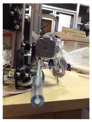
Put z screw into white plastic of extruder screw assembly. (You are looking up from what will be the bottom of the screw.) Screw into plastic piece until it starts to come out other side.
