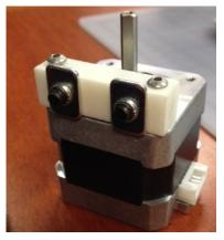
Put the piece on top of one motor such that if the motor connector is toward you, the white piece is on the left with the black line facing out and on top of the motor (the M5 black screw heads should face toward the motor center). The black line will then disappear when it is attached to the aluminum bar. The nuts should be loose so that you can slide them down the Z axis later. Set aside for now.
