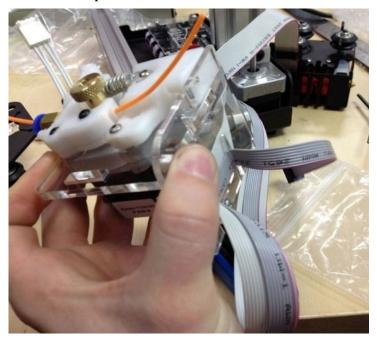
3-sided partial acrylic box around the extruder drive motor assembly.
