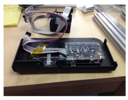
Attach the acrylic piece with the power switch to the baseplate assembly using the M5 (longer)screw and square nut and then the M3 (shorter) screw. The screw heads should face outward.
