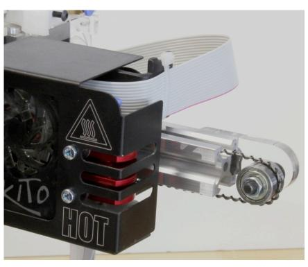
Next take the synchromesh idler (piece of acrylic with a roller) and attach it to the back of the end of the x axis. Adjust the tension of the synchromesh by pulling the idler away from the end of the x axis. Adjust the synchromesh to be tight enough so that it takes some force to tighten down the idler into position. Be sure the synchromesh isn't binding or dragging
